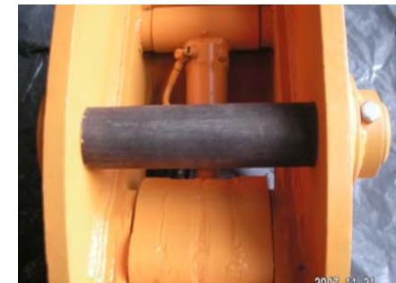
Made of steel 4140 All-hardened machine pins
