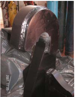
Thicker hooks, Wider carrying surface, The hooks do not open
