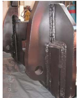
Deep drewed hooks, more support to the locking hole
