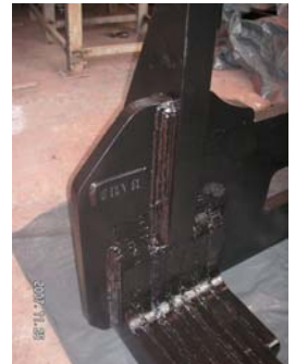
Completly supported hook – fork blade
